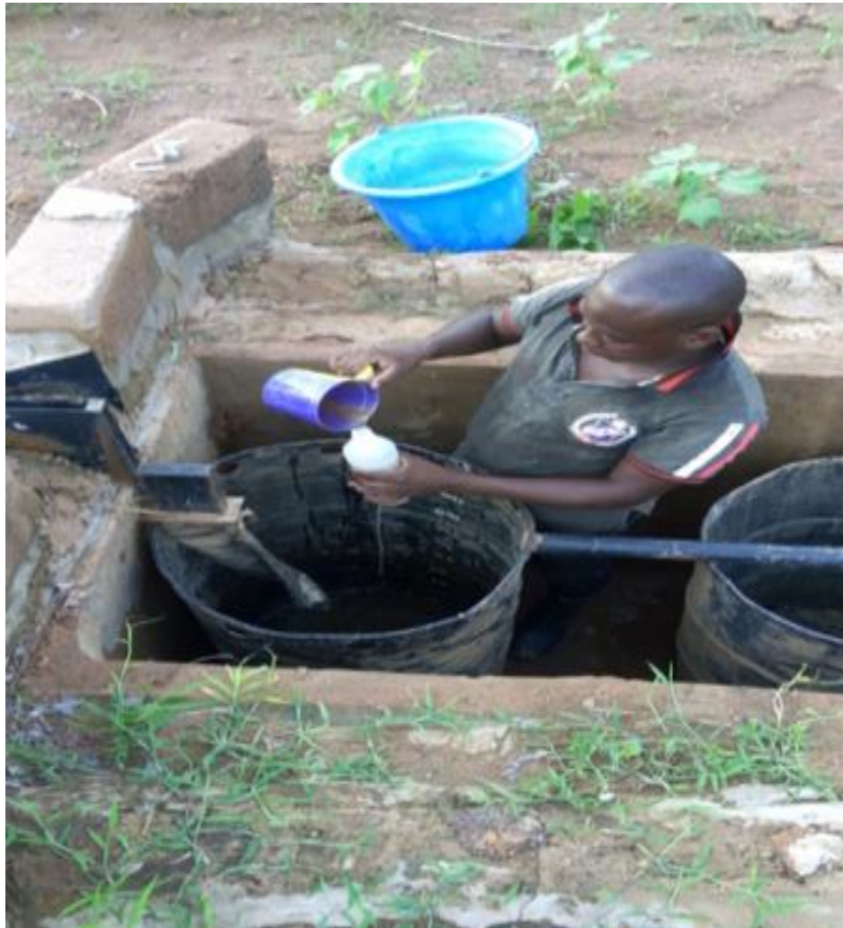
Photo 5: Device of runoff and erosion measurement at Kani
