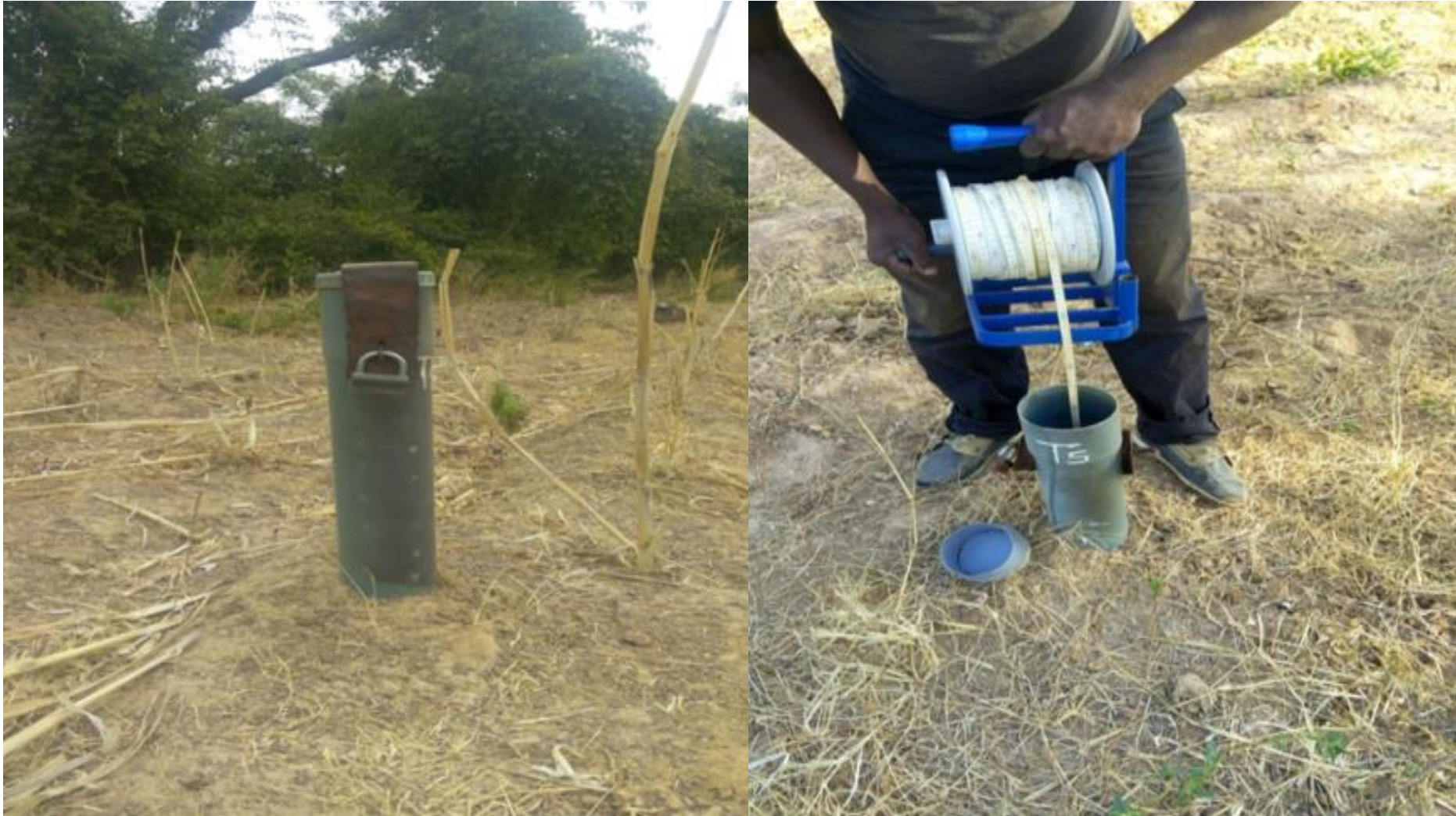
Photo 3: b) measurement of water table dynamic, a) tube protected using a padlock, Noupinesso and kani, 2018
