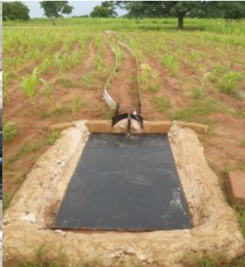
Photo 5: Device of runoff and erosion measurement at Kani
