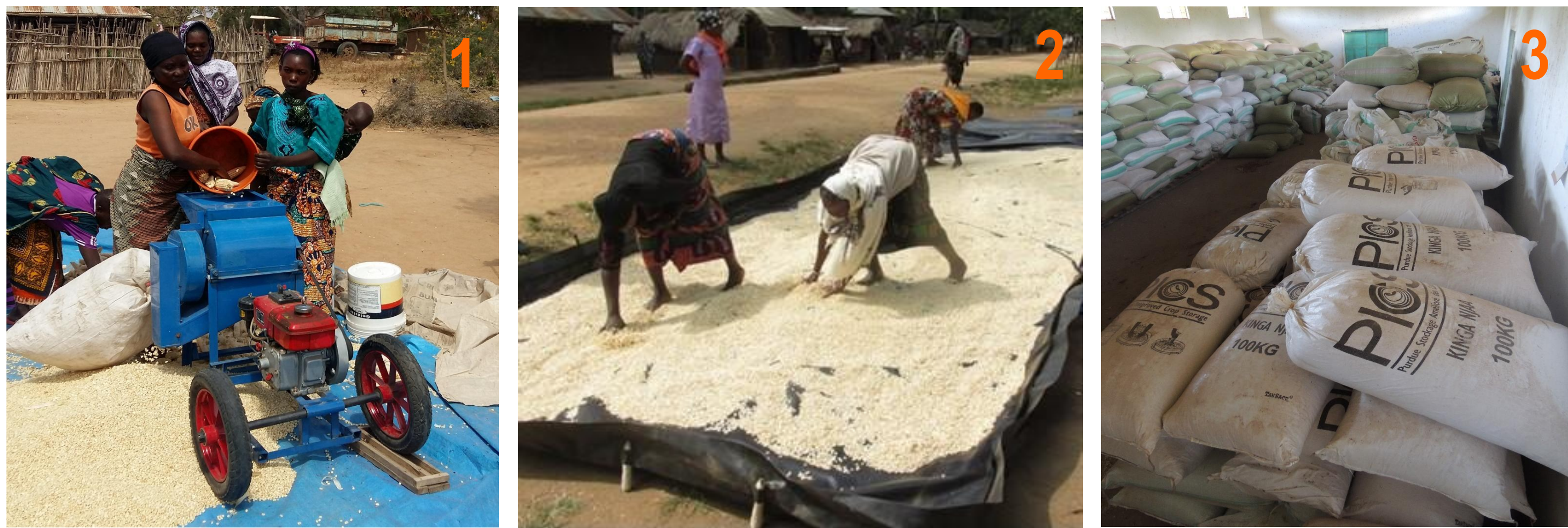
Improved postharvest technologies introduced in Tanzania: (1) mechanized maize sheller; (2) collapsible drier case; (3) hermetic storage bags.
